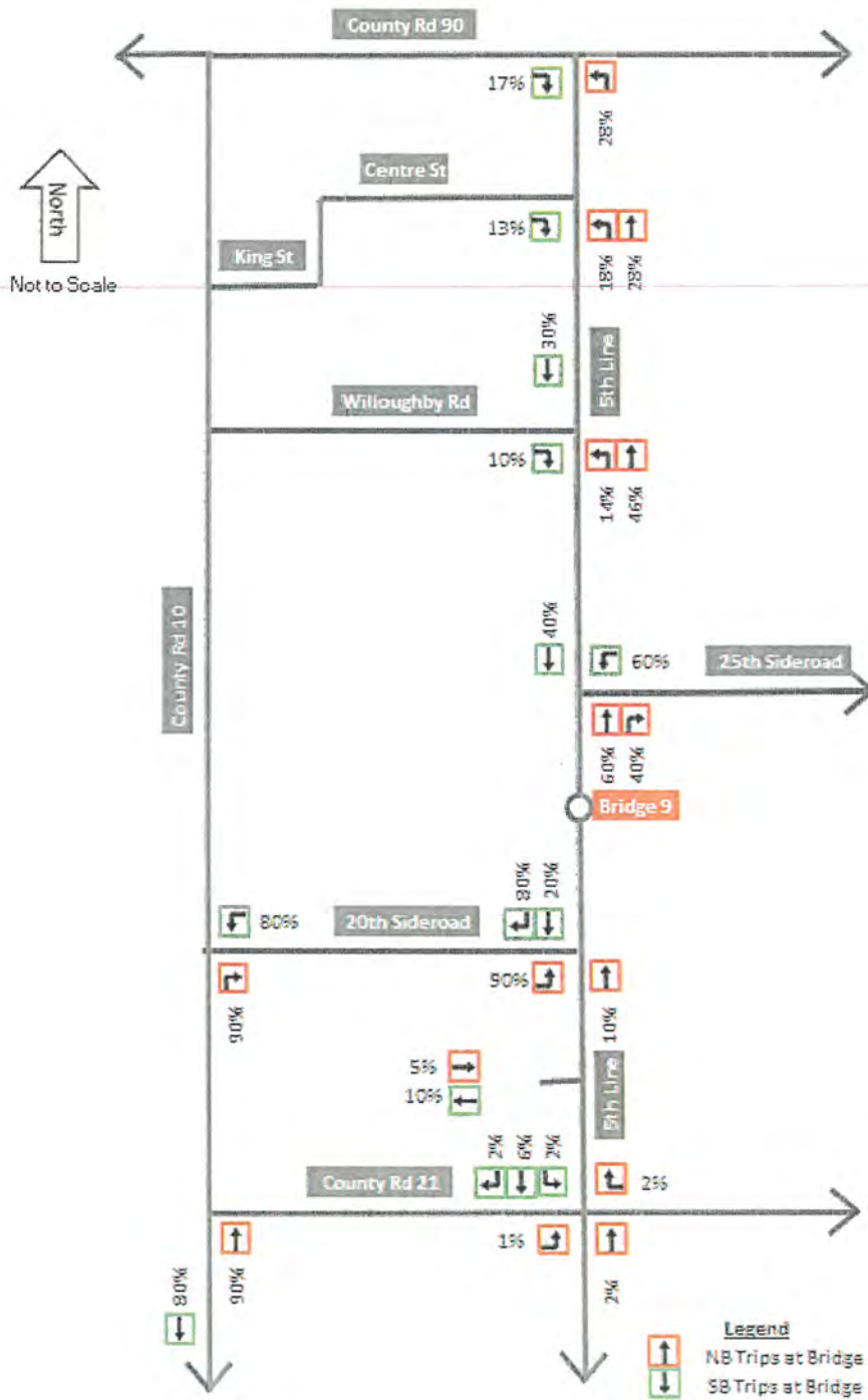
Figure 2-2. Scenario 1A - PM Peak Hour Traffic Volume Distribution of 5 th Line Bridge Traffic
