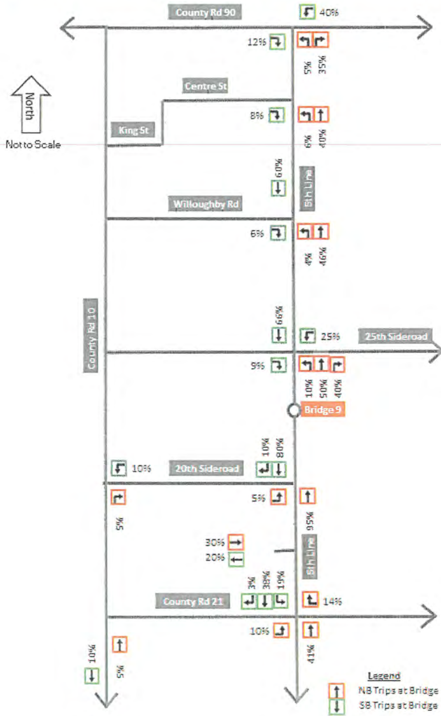
Figure 2-9. Scenario 2A - AM Peak Hour Traffic Volume Distribution of the 5th Line Bridge Traffic
