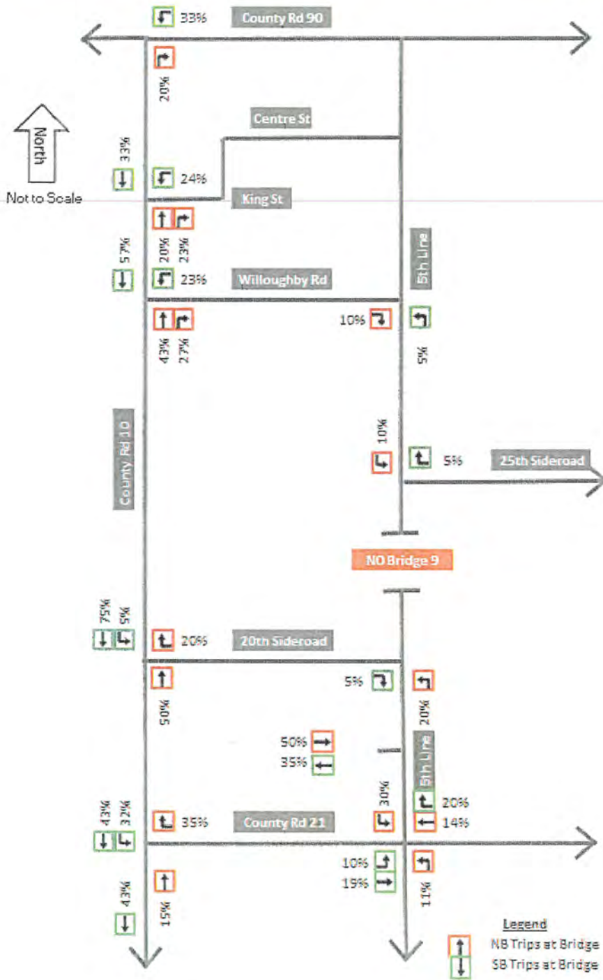
Figure 2-5. Scenario 1B - AM Peak Hour Traffic Volume Distribution of the 5 th Line Bridge Traffic
