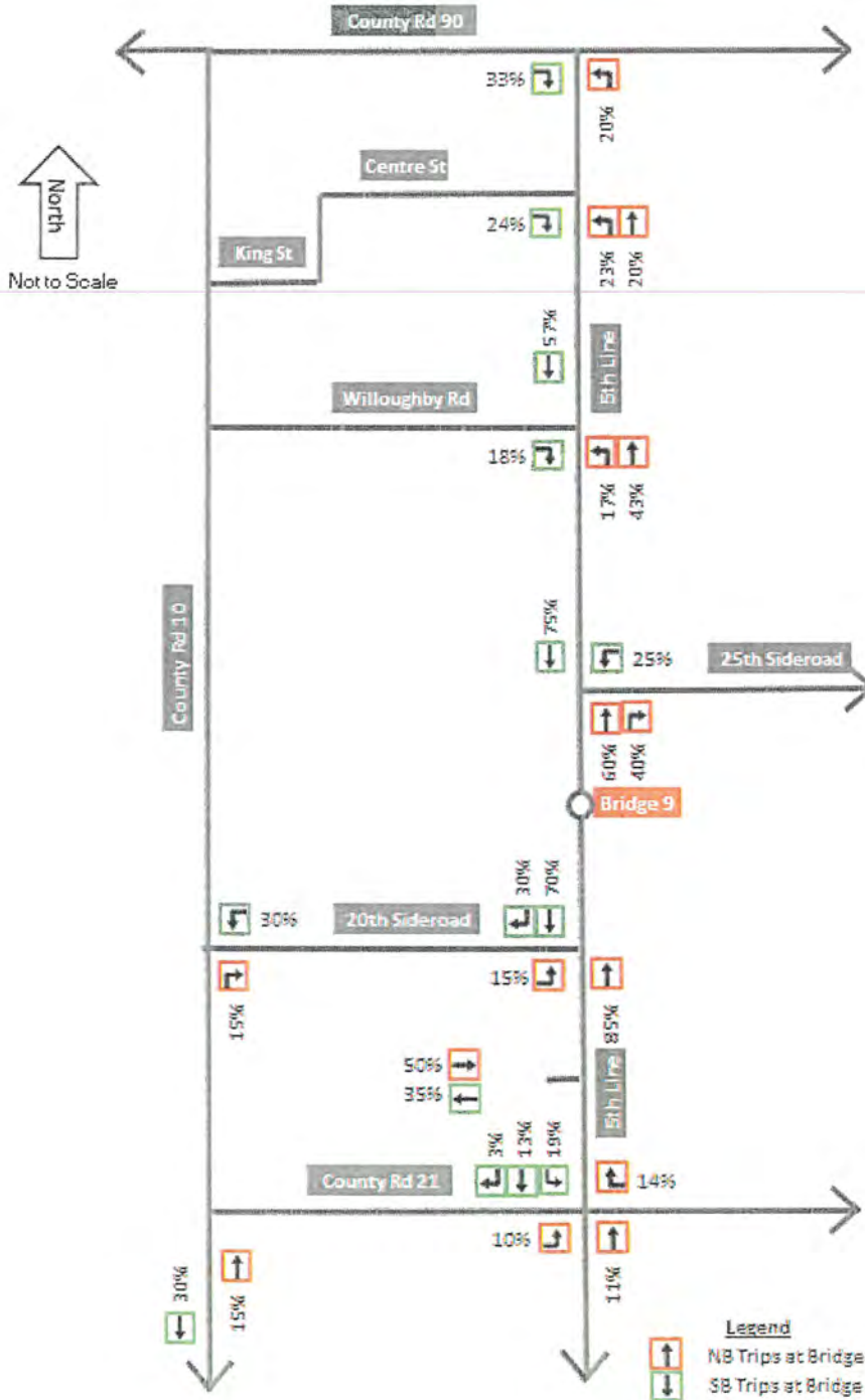
Figure 2-1. Scenario 1A - AM Peak Hour Traffic Volume Distribution of the 5 th Line Bridge Traffic
