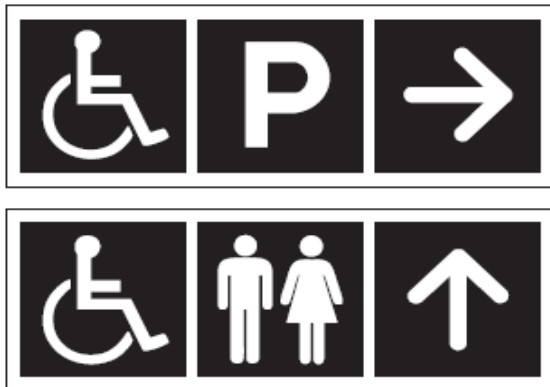
Figure A-3.8.3.1.A Signs Indicating Accessible Facilities
