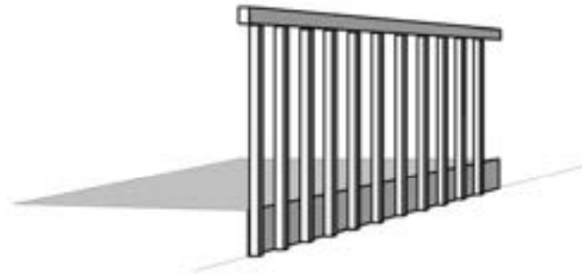
Figure A-1.2.2.B Cantilevered Picket System
